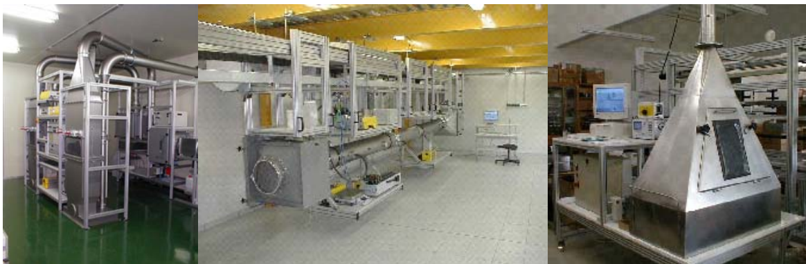
Test Rig Installation Meeting the Requirements according to DIN 71 460, EN 779 and EN 60312
